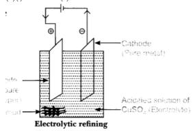
(c) Impure copper is taken as anode whereas pure copper is taken as cathode. Copper sulphate solution (CuS04) is taken as electrolyte. When electric current is passed, impure copper changes to ions which gain electrons at cathode and change into pure copper. Impurities are left behind as anode mud.
